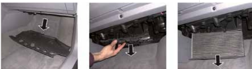
Pic. 1 - Cabin filter located behind the glove box
