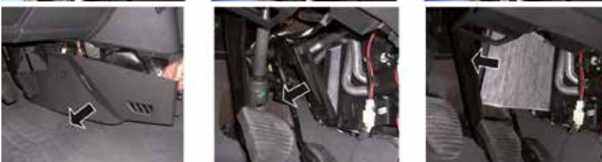
Pic. 3 - Cabin filter located near the pedals
