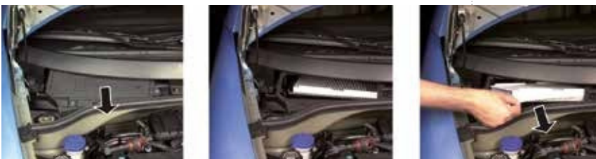
Pic. 2 - Cabin filter located behind in the engine bay, under the windshield
