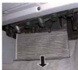
Im. 1 - Cabin filter located behind the glove box
